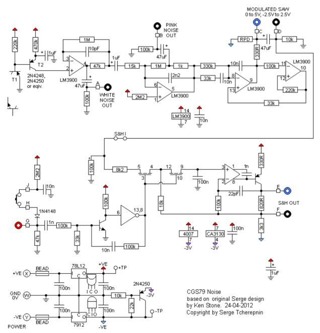
The schematic for the noise source. The upper part of the diagram shows the noise source, while the lower part shows the optional Sample and Hold. T1 at the upper left is a transistor selected for its noise characteristics. Below it is an NPN transistor shown in the orientation in which it could be used to substitute for the PNP. As only the base-emitter is used, either type of transistor will work in the circuit.
