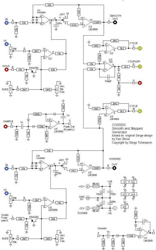
The schematic for Smooth and Stepped Generator module. Both sections are essentially identical.
