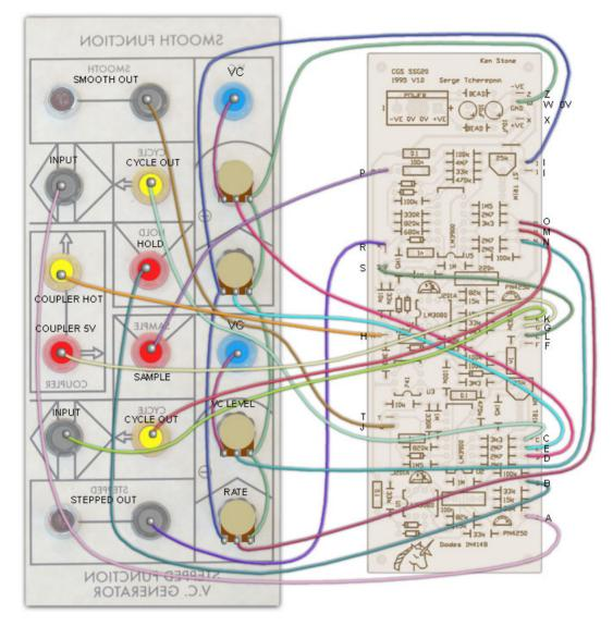
Example wiring for the Smooth and Stepped Generator.
