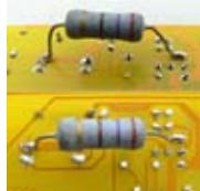
Using a 1J17B. The 1J17B is very similar to the 1J24B and can be used in its place should the 1J24B prove too hard to get. It does however use about five times as much heater current. A 270 ohm resistor soldered in as shown here (and on the circuit diagram in yellow) will provide the extra current needed. The resistor will get hot. The glow from the cathode of a 1J17B can be seen, but it is not very bright.
