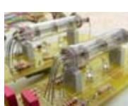
Close up of tube wiring. There is a direct relationship between the holes provided on the PCB and the positions the wires come out of the base of the tube. There is a paint spot on the tube marking pin 1, though it is not visible in this photo, as pin 1 is the furthest from us. Do **not** bend the wires at the glass, but allow a couple of millimetres at least before you bend. The 330k resistor at the lower right of the picture is the grid bias resistor referred to below.
